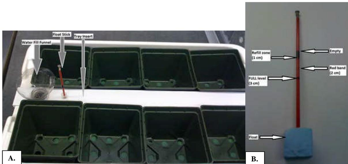
**Fig. 2 A. Image of plant tray with B. close-up of float stick for water level determination.**
